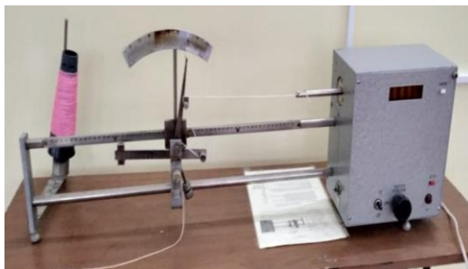
Torsion meter for measuring the degree of twisting of yarn and threads
