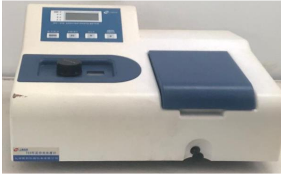
UV-Vis Spectrophotometer with a wavelength range of 325-1000 nm
