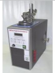
A device for measuring air permeability of 160 MT. The device is designed to measure the air permeability of textile materials, paper and cardboard, building materials, etc., and is used in testing laboratories of various enterprises.
