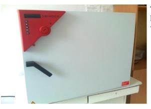
The drying Cabinet is used for determining the humidity of bakery products and drying after washing chemical dishes
