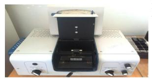
Photoelectrocolorimeter apparatus for testing drinking water samples
