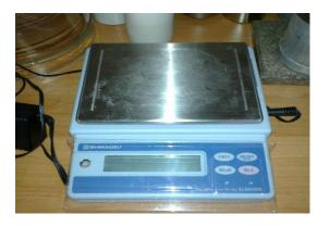
Analytical scales XA 220 / y-Scales are designed for accurate weighing in the laboratory.It is designed for automatic measurement, the product must be properly packaged manually or placed in the center of the measuring container.
